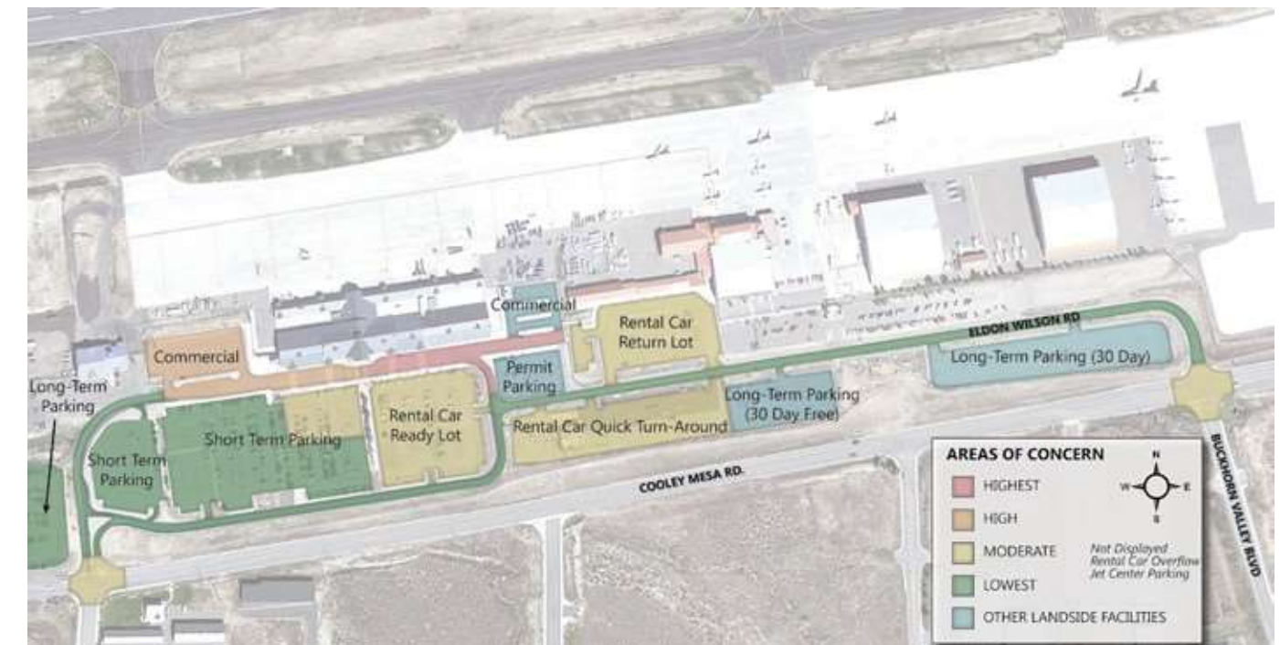
FIGURE 1.13 LANDSIDE/ROADWAY SYSTEM OVERVIEW AND AREAS OF CONCERN
